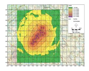
The noise map can then be easily compared with the results of the baseline noise survey to determine compliance with criteria contained in the Guidelines for Planning Authorities June 2006 – Wind Energy Development Guidelines.
